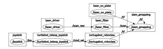
Figure 5 The computational graph of Tortugabot from the minimal\_laser.launch and gmapping.launch files. Each box in the graph is an individual node. The strings on the arrows are topics being broadcast and listened to by each node.
