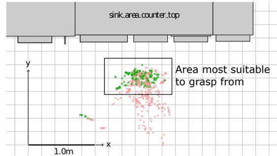
**Fig. 6:** Robot base poses from episodes during which the robot succeeded (indicated by green dots), and failed (indicated by red dots) to grasp a cup from the counter top of a sink.
