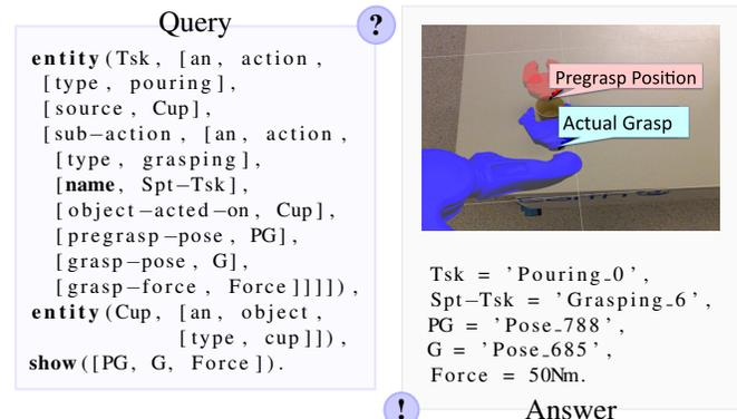
**Fig. 2:** A typical query in KNOWROB2 on the left, and the inferred answer shown in OPENEASE on the right side.
