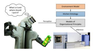
Fig. 1. Application of models representing organizational principles on a robot system: The robot acquires models given observations of the objects found within its environment. In order to determine a suitable storage location for a given object, it identifies the class to which the object belongs and performs inference over the model using, in particular, features pertaining to the similarity between the object and the other objects already stored in the environment.
