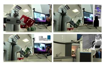
Fig. 10. Pictures of the live demonstration: The robot empties the shopping basket and identifies the categories to which the items belong. It then infers a suitable storage location given its knowledge of the environment and places the object accordingly.
