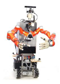
Fig. 1. TUM-Rosie, our mobile manipulation platform. Fingertip sensors installed in its right hand improve autonomous grasping, let it recognize object surfaces, and detect object slip.
