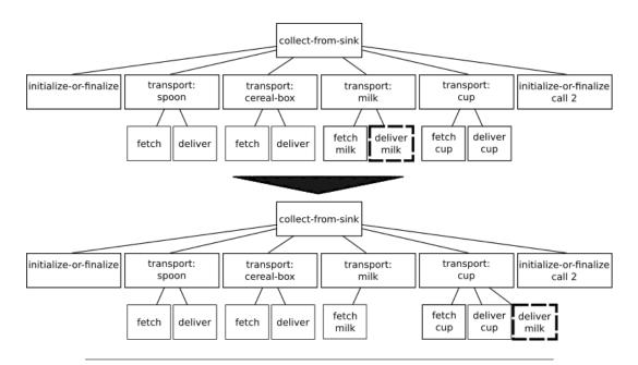
FIGURE 3.7: Scenario 1 task tree transformed with both-hands-rule. It delays one *delivery* action to be executed after the second transport.
