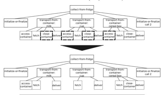
FIGURE 3.10: Scenario 2 task tree transformed with environmentrule. It skips opening and closing containers between the first *access-container* and the last *closing-container* action
