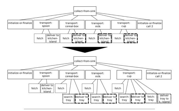
FIGURE 3.8: Scenario 1 task tree transformed with tray-rule. The rule changes the delivery location of up to three objects to a pose on the tray and appends a *fetching* and *delivering* action for the tray.
