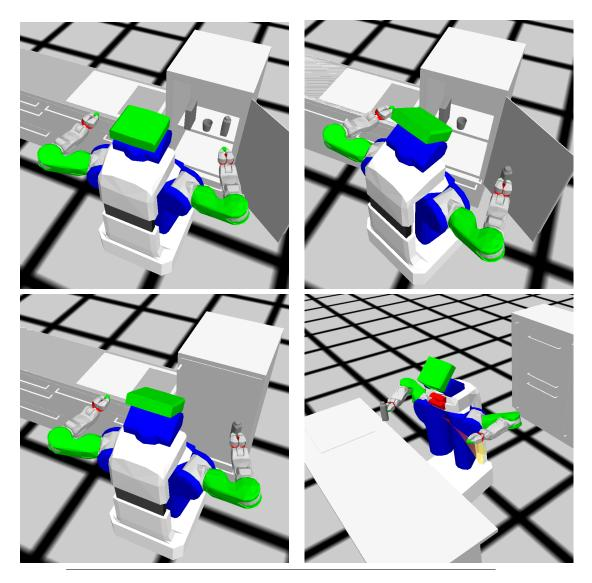
FIGURE 3.3: Scenario 2. (top left) Open the fridge to see three objects inside, (top right) fetch the milk, (bottom left) close the fridge door and (bottom right) deliver the object onto the kitchen island.
