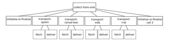
FIGURE 3.4: Scenario 1 task tree, transporting four objects with initializing and finalizing the plan.
