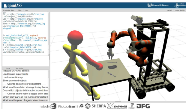
Fig. 7. The OPENEASE [17] online knowledge processing system allows reviewers and readers to independently analyse the data logged in our experiments. Semantic queries using the descriptions of objects, humans, motions, and events show how safety-aware robotic agents could make sense of their low-level percepts using these concepts.
